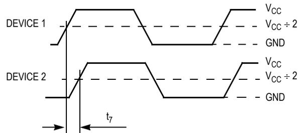
Figure 4. Device-to-Device Skew
