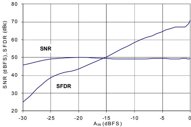
FIGURE 5. SNR AND SFDR vs A<sub>IN</sub>
