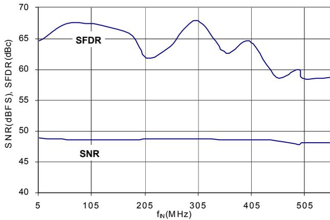
FIGURE 3. SNR AND SFDR vs f<sub>IN</sub>
