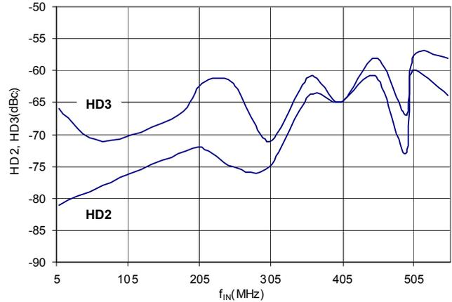
FIGURE 4. HD2 AND HD3 vs f<sub>IN</sub>
