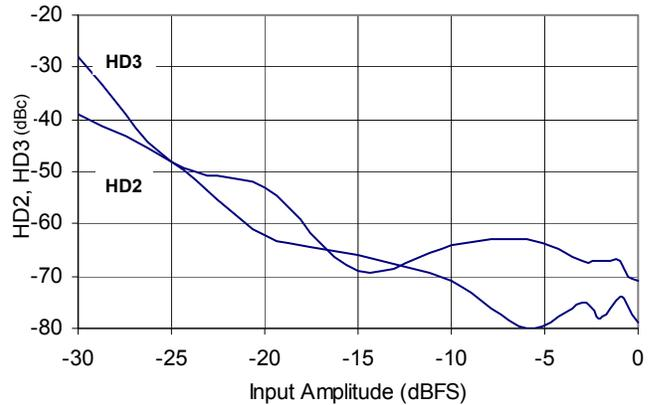
FIGURE 6. HD2 AND HD3 vs A<sub>IN</sub>
