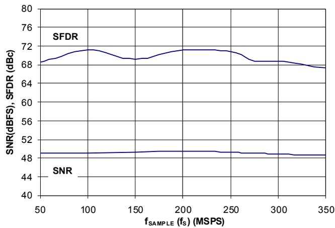
FIGURE 7. SNR AND SFDR vs f<sub>SAMPLE</sub>
