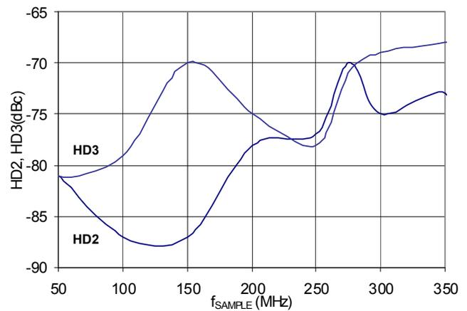
FIGURE 8. HD2 AND HD3 vs f<sub>SAMPLE</sub>
