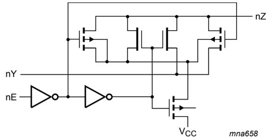
Figure 3. Logic diagram (one switch)
