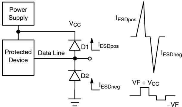
Looking at the figure above, it can be seen that when a positive ESD condition occurs, diode D1 will be forward biased while diode D2 will be forward biased when a negative ESD condition occurs. For slower transient conditions, this system may be approximated as follows:
