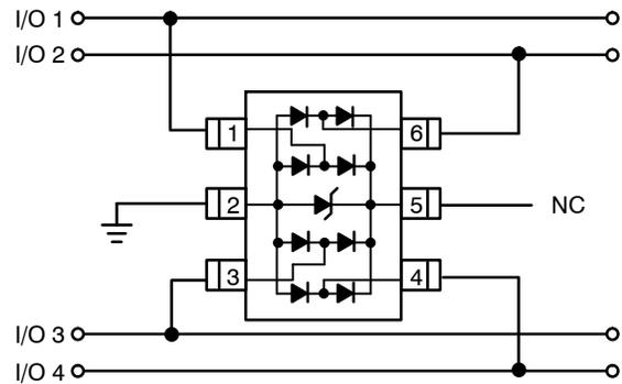
In applications lacking a positive supply reference or those cases in which a fully isolated power supply is required, the internal TVS can be used as the reference. For these applications, pin 5 is not connected. In this configuration, the steering diodes will conduct whenever the voltage on the protected line exceeds the working voltage of the TVS plus one diode drop ( $V_C = V_f + V_{TVS}$ ).
