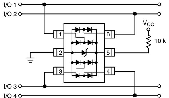
The NUP4114 can be isolated from the power supply by connecting a series resistor between pin 5 and  $V_{CC}$ . A 10 kΩ resistor is recommended for this application. This will maintain a bias on the internal TVS and steering diodes, reducing their capacitance.
