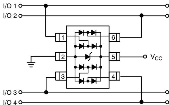
For this configuration, connect pin 5 directly to the positive supply rail ( $V_{CC}$ ), the data lines are referenced to the supply voltage. The internal TVS diode prevents overvoltage on the supply rail. Biasing of the steering diodes reduces their capacitance.
