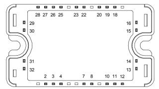
All multiple inputs and outputs must be shorted together Example: 13/14; 29/30; 22/23 ...
