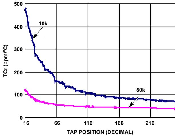
FIGURE 11. TC FOR RHEOSTAT MODE IN ppm
