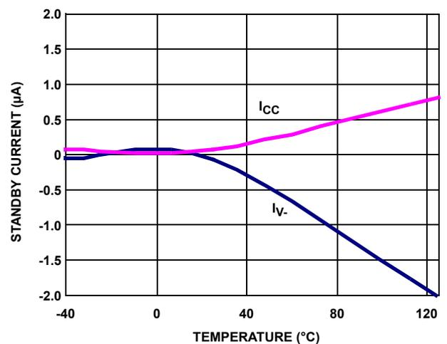
FIGURE 2. STANDBY  $I_{CC}$  and  $I_{V-}$  vs TEMPERATURE
