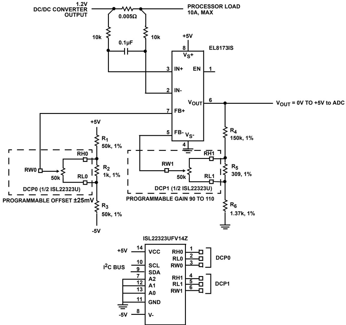
FIGURE 20. CURRENT SENSING WITH GAIN AND OFFSET CONTROL
