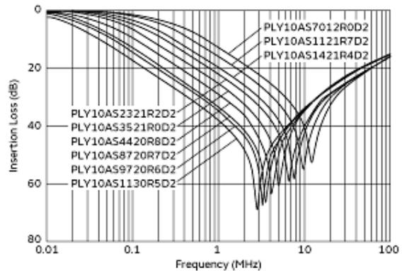
Differential Mode Insertion Loss-Frequency Characteristics
