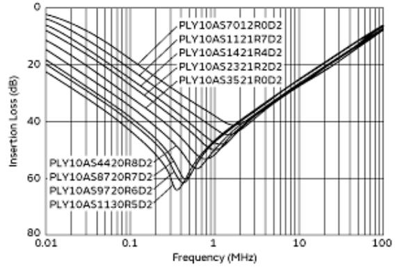
Common Mode Insertion Loss-Frequency Characteristics
