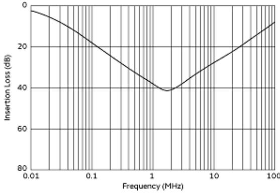
Common Mode Insertion Loss (Typ.)
