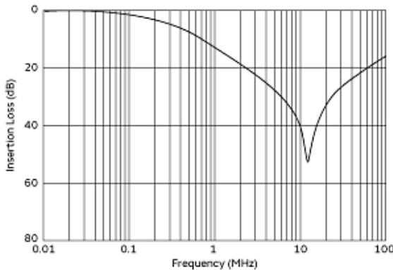
Differential Mode Insertion Loss (Typ.)
