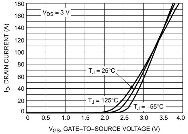
Figure 2. Transfer Characteristics
