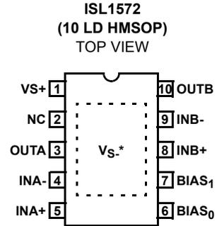
\*THERMAL PAD MUST BE CONNECTED TO NEGATIVE SUPPLY:  $V_{S-}$ .
