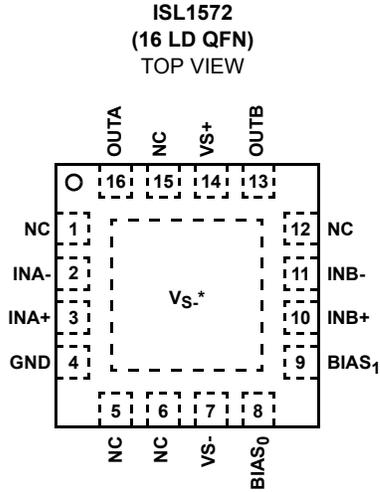
\*THERMAL PAD MUST BE CONNECTED TO NEGATIVE SUPPLY:  $V_{S-}$ .
