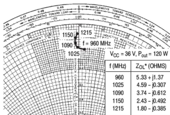
Z<sub>OL</sub>\* = Conjugate of the optimum load impedance into which the device output operates at a given output power, voltage and frequency.
