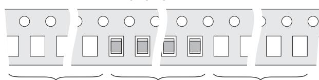
230mm min.-560mm max. May consist of carrier and/or cover tape followed by a minimum of 160mm of carrier with sealed cover tape
