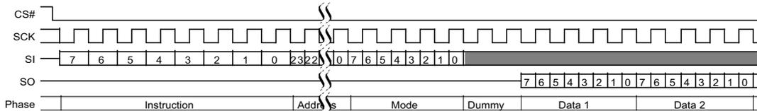
**Figure 84. Continuous DDR Fast Read Subsequent Access (3-Byte Address [ExtAdd=0, EHPLC=11b])**
