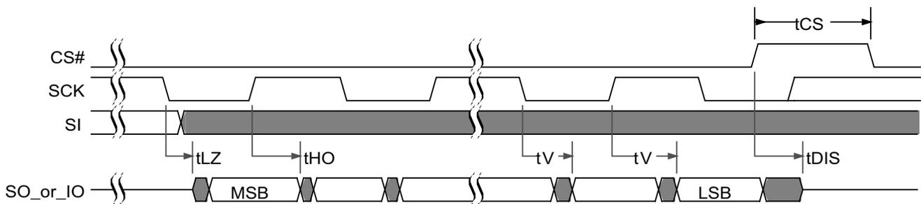
Figure 38. SPI DDR Data Valid Window
