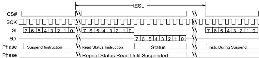
**Figure 102. Erase Resume (ERRS 7Ah) Command Sequence**
