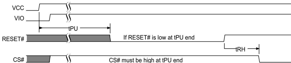
Figure 27. Reset High at the End of POR
