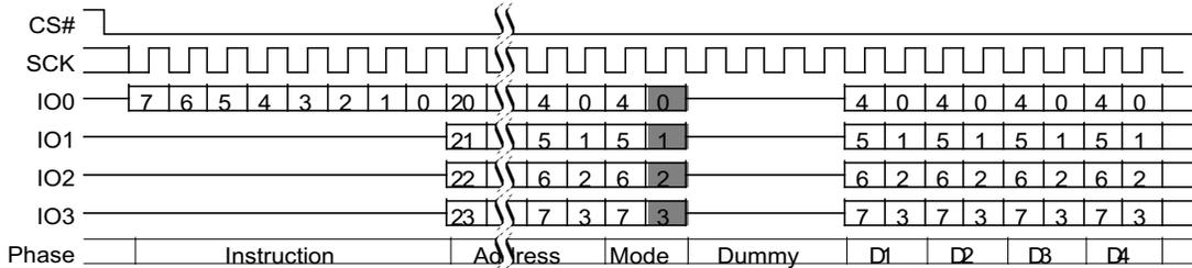
**Figure 80. Continuous Quad I/O Read Command Sequence (3-Byte Address), LC=00b**
