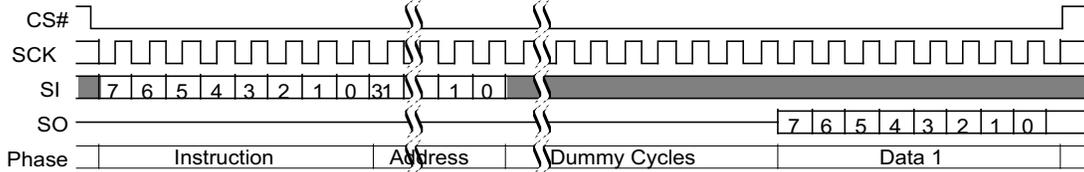
Figure 12. Dual Output Command
