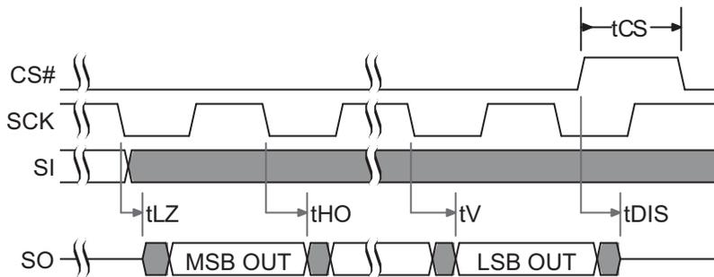
Figure 33. SPI SDR MIO Timing
