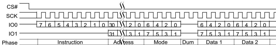
Figure 78. Continuous Dual I/O Read Command Sequence (4-Byte Address, BCh or BBh [ExtAdd=1], EHPLC=10b)
