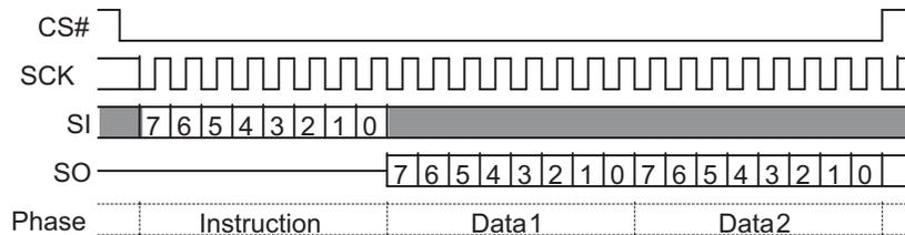
Figure 10. Single Bit Wide I/O Command without Latency
