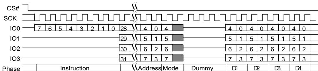
Figure 16. DDR Fast Read with EHPLC = 00b
