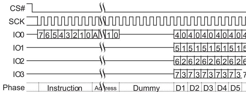
**Figure 74. Quad Output Read (QOR 6Bh or 4QOR 6Ch) Command Sequence without Read Latency**
