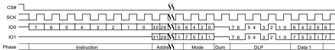
**Figure 89. Continuous DDR Dual I/O Read Subsequent Access (4-Byte Address, EHPLC= 01b)**
