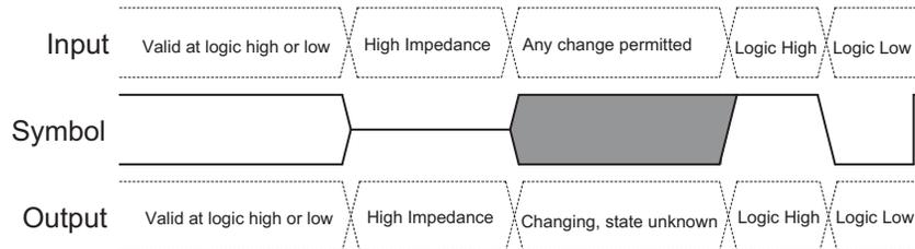
Figure 24. Input, Output, and Timing Reference Levels
