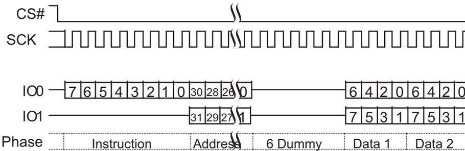
Figure 77. Dual I/O Read Command Sequence (4-Byte Address, BCh or BBh [ExtAdd=1], EHPLC=10b)
