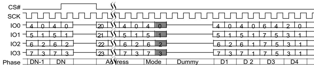
**Figure 81. Quad I/O Read Command Sequence(4-Byte Address, ECh or EBh [ExtAdd=1], LC=00b)**
