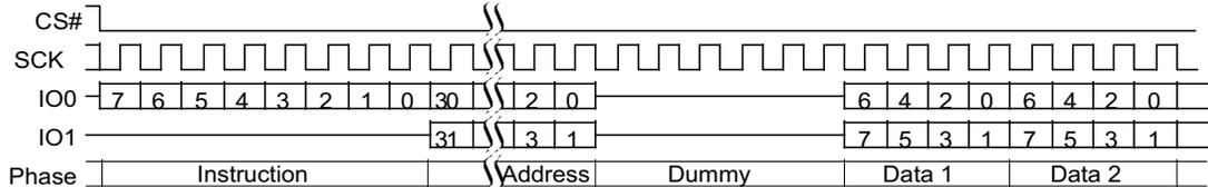
Figure 15. Quad I/O Command
