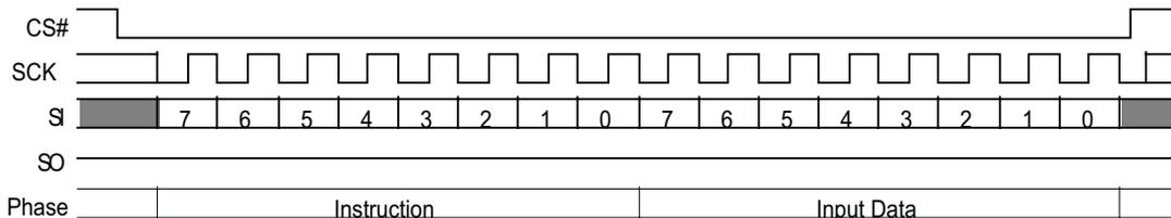
Figure 9. Single Bit Wide Output Command
