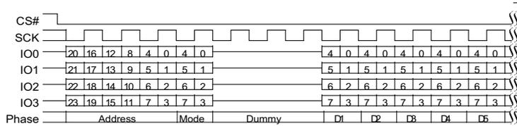
**Figure 93. DDR Quad I/O Read Initial Access (4-Byte Address, EEh or EDh [ExtAdd=1], EHPLC=01b)**
