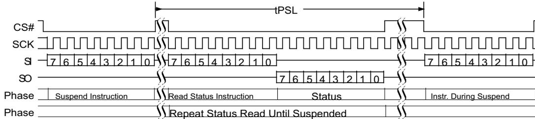
Figure 98. 10.55 Program Resume (PGRS 8Ah) Command Sequence
