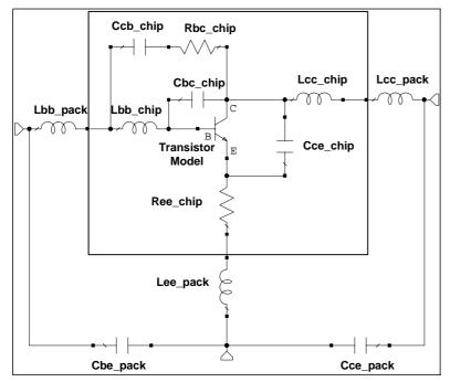
0.212 nΑ  $L_{\rm bb\_chip} =$ 0.07472  $L_{\rm cc\ chip} =$ nΗ 0.0184  $L_{\rm bb\_pack} =$ nΗ nΗ  $L_{\text{cc\_pack}} =$ 0.277 nΗ 0.239  $L_{\text{ee}\_\text{pack}} =$ 0.015 рF  $C_{\rm bc\ chip} =$ 0.013 pF  $C_{\text{cb\_chip}} =$ 0.282  $C_{\text{ce\_chip}} =$ pF 0.064 pF C<sub>be pack</sub> = 0.0492 pF  $C_{\text{ce\_pack}} =$ 7 Ω  $R_{\rm bc\ chip} =$ 0.566 Ω  $R_{\text{ee chip}} =$ Valid up to 6GHz
