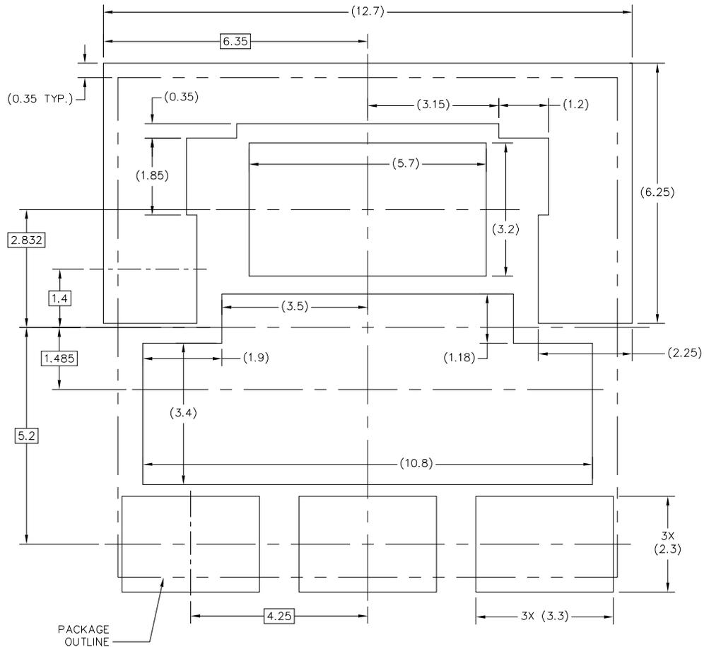
PCB DESIGN GUIDELINES – SOLDER MASK OPENING PATTERN 2
