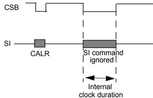
If the negative CSB pulse is outside a predefined time range (from  $t_{CSB(MIN)}$  to  $t_{CSB(MAX)}$ ), the calibration event will be ignored and the internal clock will be unaltered or reset to its default value ( $f_{PWM(0)}$ ) if this was not calibrated before.
