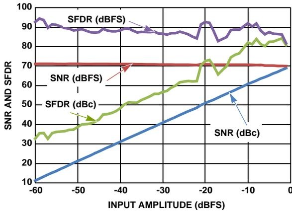
FIGURE 4. SNR AND SFDR vs A<sub>IN</sub>
