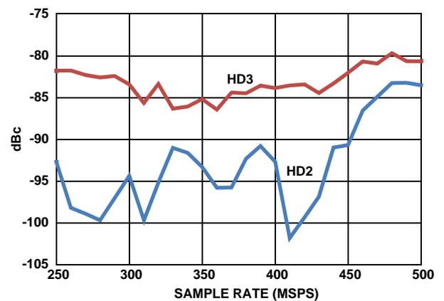
FIGURE 7. HD2 AND HD3 vs f<sub>SAMPLE</sub>
