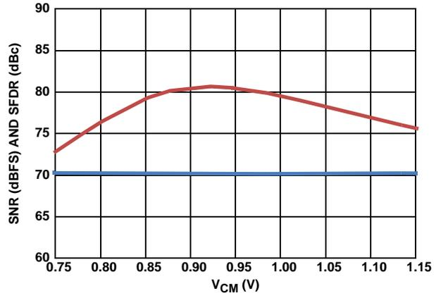
FIGURE 11. SNR AND SFDR vs V<sub>CM</sub>
