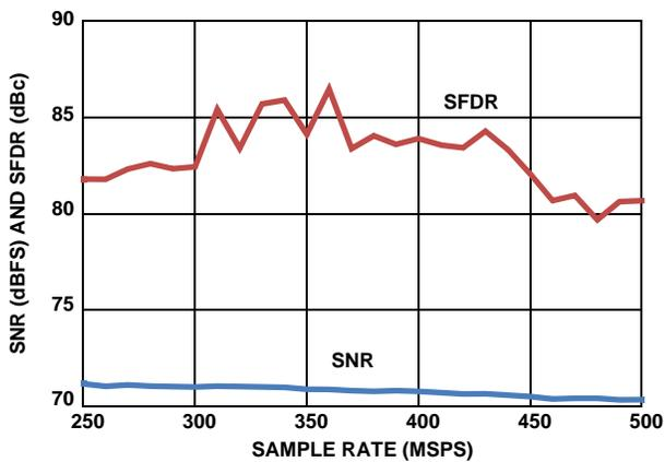
FIGURE 6. SNR AND SFDR vs f<sub>SAMPLE</sub>
