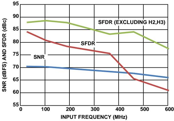
FIGURE 2. SNR AND SFDR vs f<sub>IN</sub>
