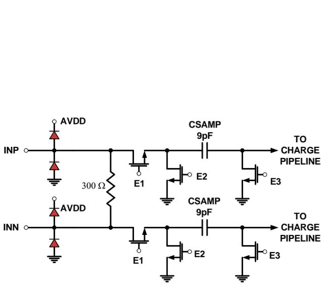
FIGURE 43. ANALOG INPUTS
