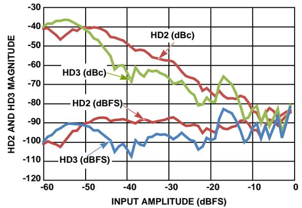
FIGURE 5. HD2 AND HD3 vs A<sub>IN</sub>
