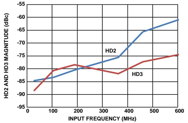
FIGURE 3. HD2 AND HD3 vs f<sub>IN</sub>
