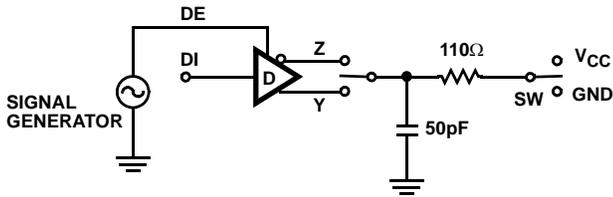
FIGURE 3A. TEST CIRCUIT
