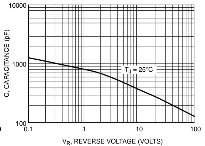
**Figure 8. Typical Capacitance**
