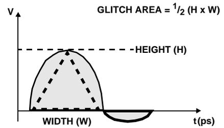
FIGURE 3. PEAK GLITCH AREA (SINGLET) MEASUREMENT METHOD
