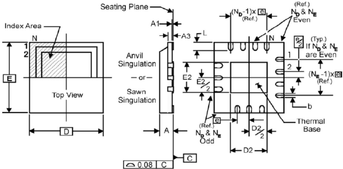
NOTE: The following package mechanical drawing is a generic drawing that applies to any pin count VFQFN package. This drawing is not intended to convey the actual pin count or pin layout of this
