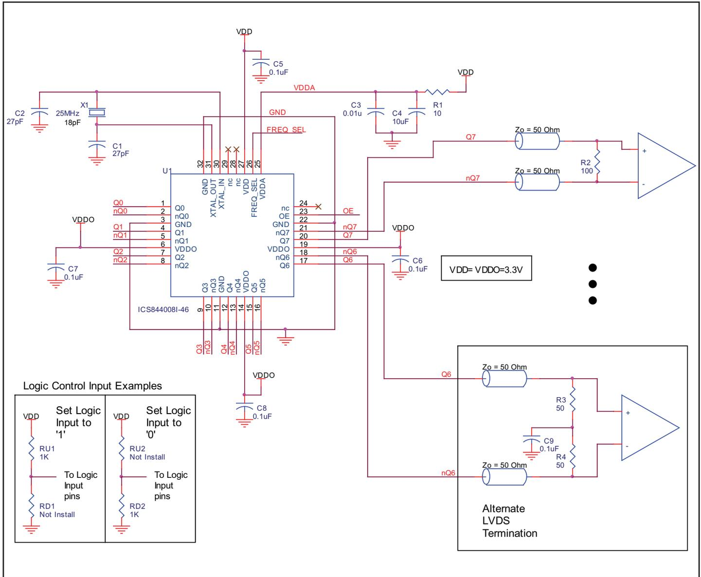
FIGURE 6. 8440081-46 SCHEMATIC LAYOUT
