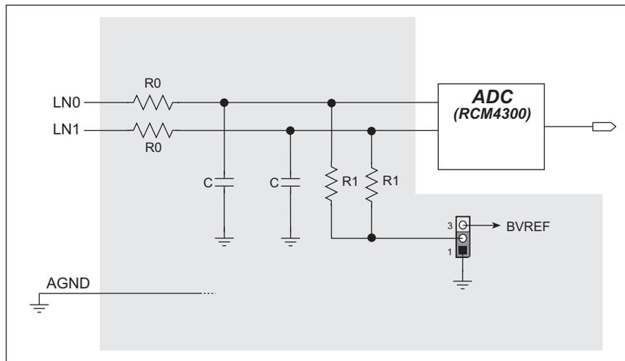
**Figure 10. Resistor Divider Network for Analog Inputs**
