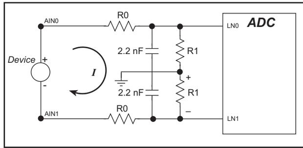
**Figure 11. Current Flow from Ungrounded or Floating Source**
