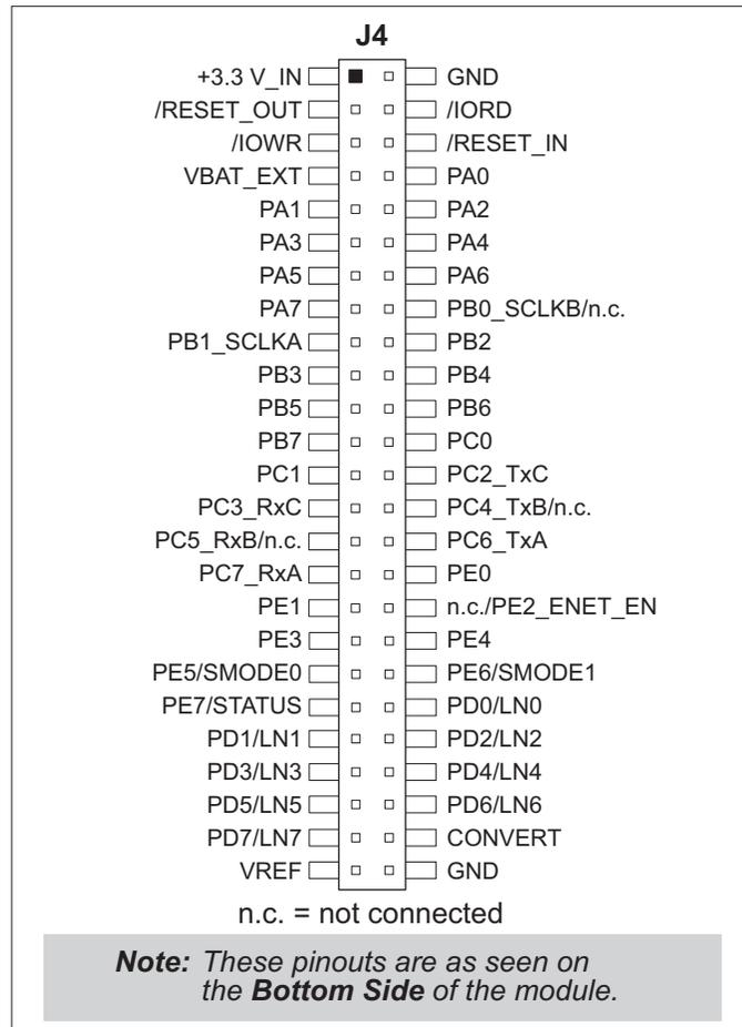
**Figure 6. RCM4300 Pinout**
