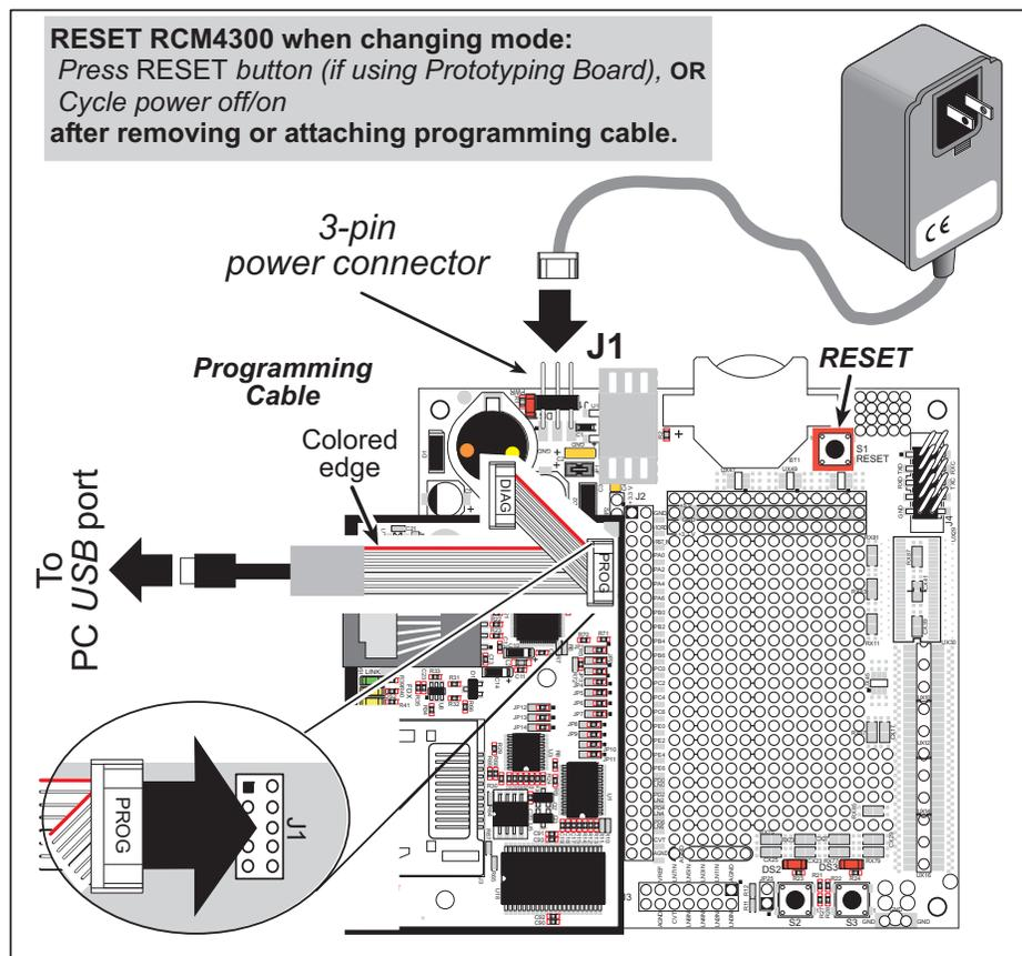
**Figure 9. Switching Between Program Mode and Run Mode**
