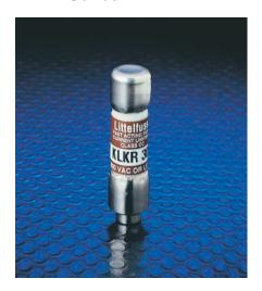
KLKR series Class CC fuses are fastacting fuses intended for general purpose branch circuit protection. Their compact size, fast-acting overload response, and their highly current limiting design make them ideal for use in OEM equipment and control panels. Solid-state devices such as SCRs and other electronic equipment generally require fast-acting protection.
