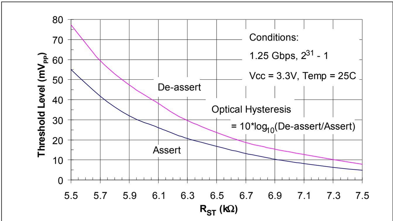
Figure 4-3. Typical Loss of Signal Characteristic (Low Input Signal Range)
