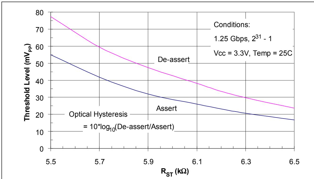
Figure 4-5. Typical Loss of Signal Hysteresis Characteristic (Full Input Signal Range)
