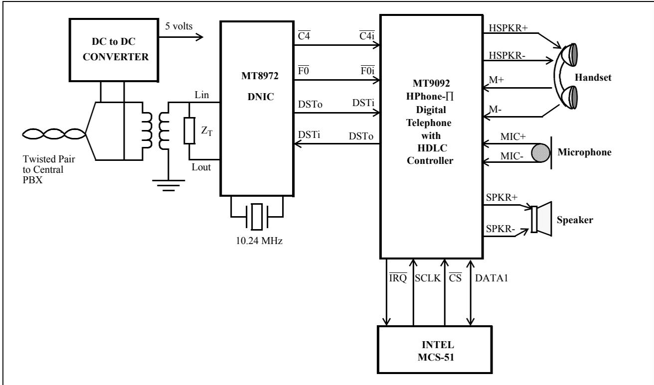
Figure 11 - Voice/Data Digital Telephone Set Circuit
