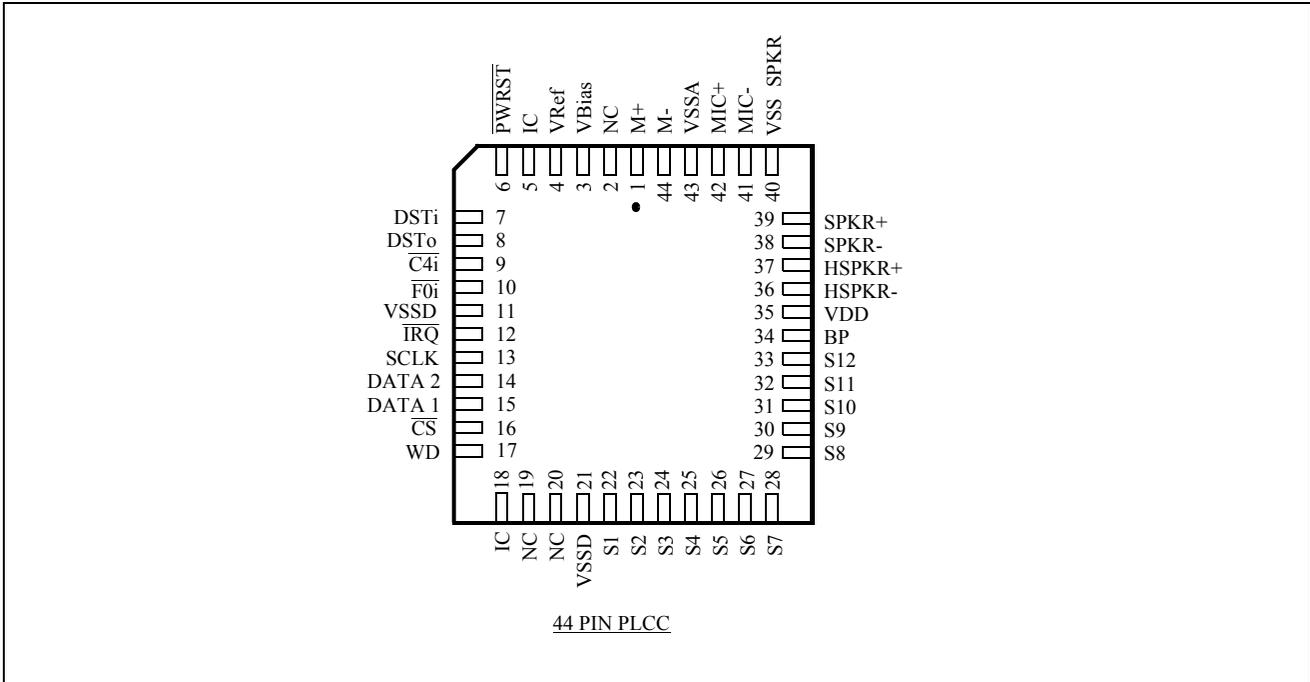
Figure 2 - Pin Connections
