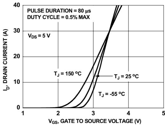
**Figure 5. Transfer Characteristics**
