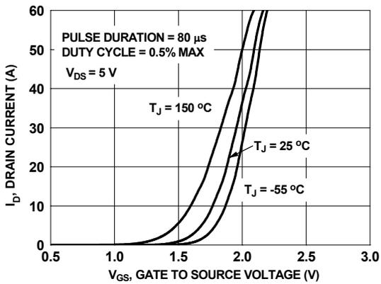
Figure 5. Transfer Characteristics
