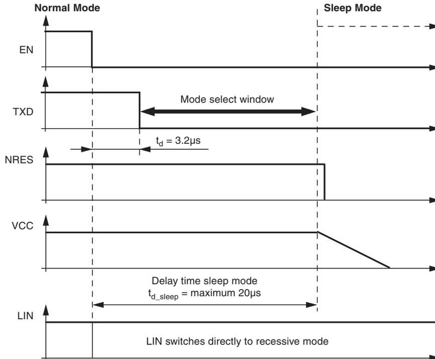
**Figure 4-5. LIN Wake-up Diagram from Sleep Mode**
